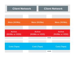
Cold Storage is a low-cost S3 Glacier-compatible storage class based on Quantum's RAIL Architecture (Redundant Array of Independent Libraries) and patented\* two-dimensional erasure coding (2D EC). 2D EC distributes object shards within and across tapes, drives, libraries, and data centers, simultaneously maximizing performance, durability, and efficiency. ActiveScale Cold Storage inherits tape's outstanding economics, reliability, and security, while dramatically simplifying tape management.
