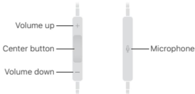
In the following instructions, ● indicates a quick press of the center button and ■ indicates a press and hold of the center button. When doing multiple presses, make sure they quickly follow one another.
