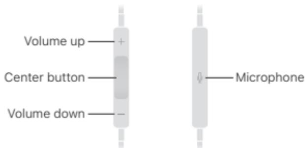
In the following instructions, ● indicates a quick press of the center button and ■ indicates a press and hold of the center button. When doing multiple presses, make sure they quickly follow one another.
