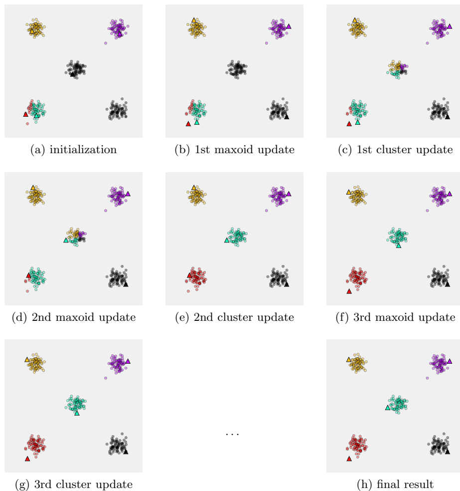
Fig. 3: Convergence behavior of k -maxoid clustering applied to a 2D data set containing five blob like clusters. Started with a random initialization of maxoids, the algorithm quickly moves them apart and converges within four iterations.
