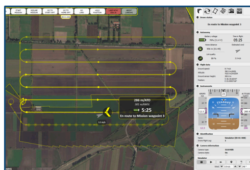
Fig. 8. UAV flight control monitor
