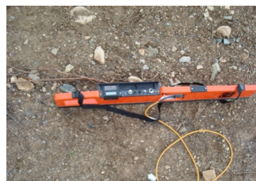
Fig. 2. Electromagnetic induction (EM) instrument.
