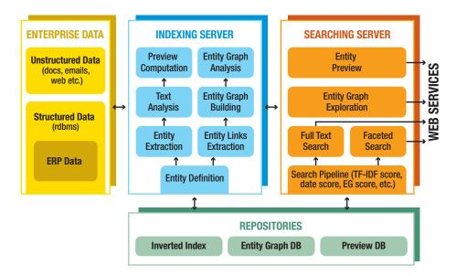
Fig. 1. Overview of the architecture of SeNSE.
