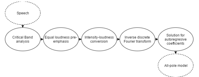
Fig. 1. Calculating perceptual linear prediction cepstral coefficients.
