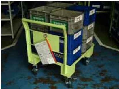
Fig. 5. RFID-tag attached to Job order sheet
