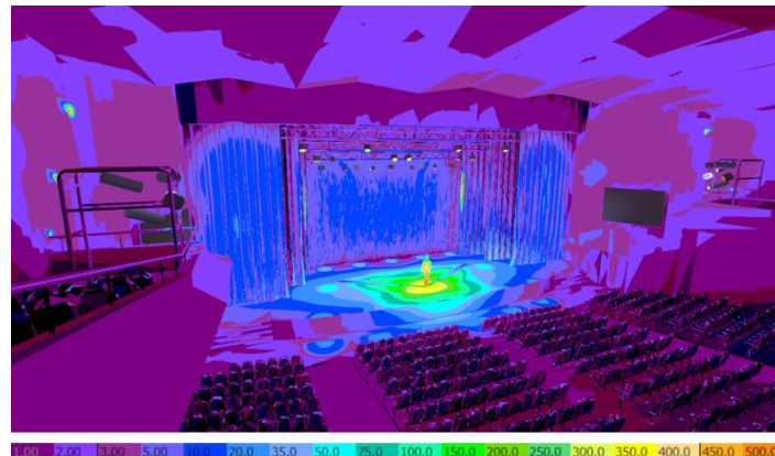
Fig. 8. Illumination model of the auditorium of NUST “MISIS” (presenter’s speech)
