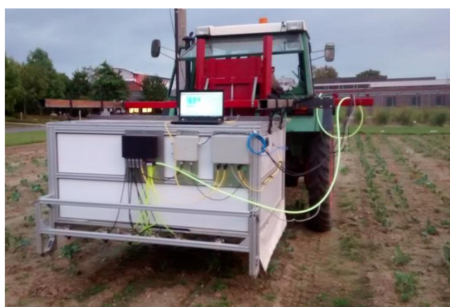
Figure 11.5 - VisionSpray mounted on a tractor.
