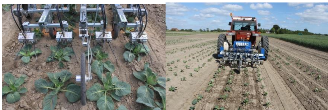
Figure 4.1 - Robotic weeding with Robovator in Denmark
