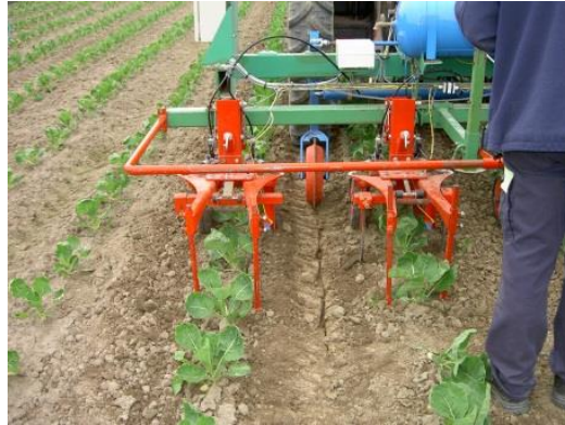
Figure 4.2 - Robotic weeding with Radis 2.0 in the Netherlands
