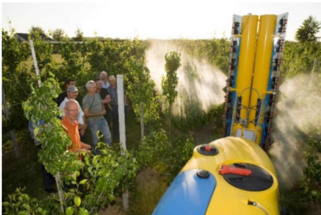
Figure 11.4 - The Canopy Density Sprayer for pomefruit trees.
