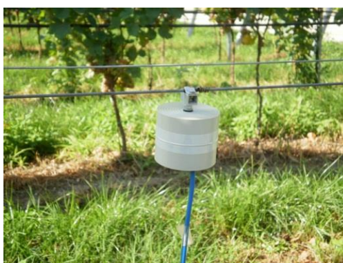
Figure 11.3 - Electromagnetic shaker for mating disruption of Scaphoideus titanus in grapevine.
