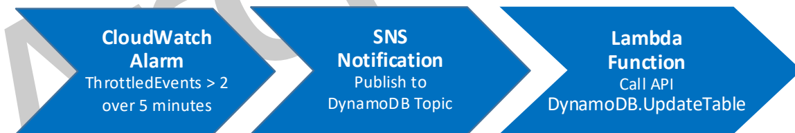
Figure 6: Example of a CloudWatch alarm flow
