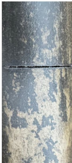
3.5 in. pipe retrieved to surface with 2.7 in. slot created.
