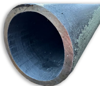
Clean electro-mechanical cut finish when pipe retrieved to surface.
