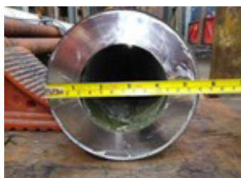
Images of the retrieved 5.5 in. heavy weight drill pipe with 1.125 in. wall thickness at surface following successful cut
