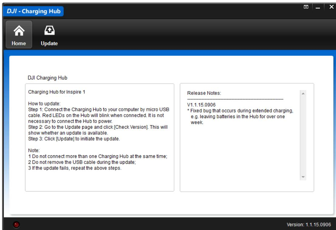
3. Connect the Charging Hub to a computer using a Micro USB cable. The bottom left indicator glows green after it is successfully connected.
