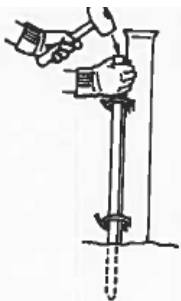
Fig. 4: Insert white oak stake into the two ties and drive into the ground until the top of the stake is 2-3" above the top tie.
