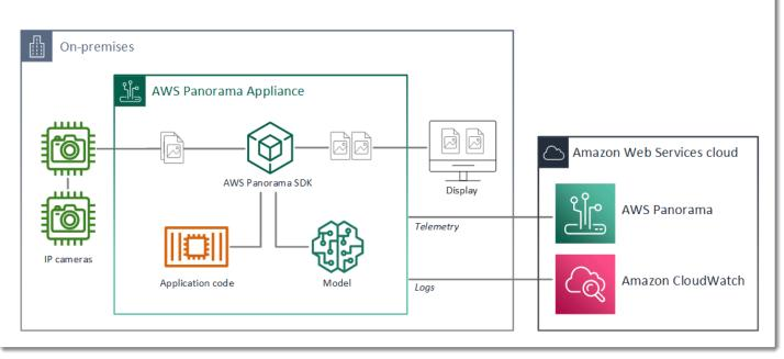
In this example, the application uses the AWS Panorama Application SDK to get frames of video from a camera, preprocess the video data, and send the data to a computer vision model that detects objects. The application displays the result on an HDMI display connected to the appliance.
