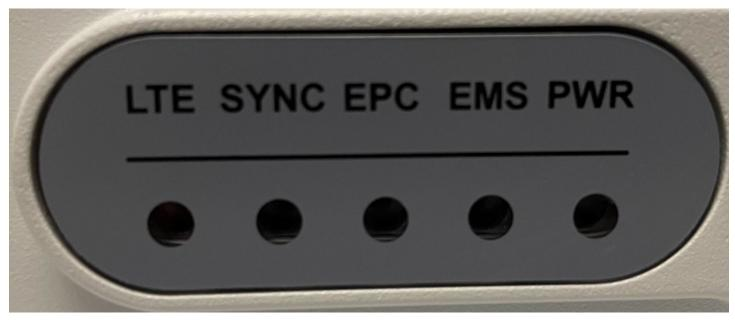
The following is a picture of the light panel on a radio unit.
