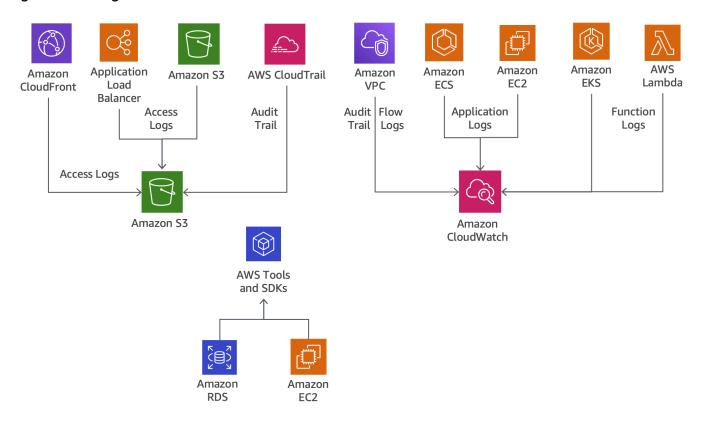
Figure 12: Logging capabilities of AWS services
