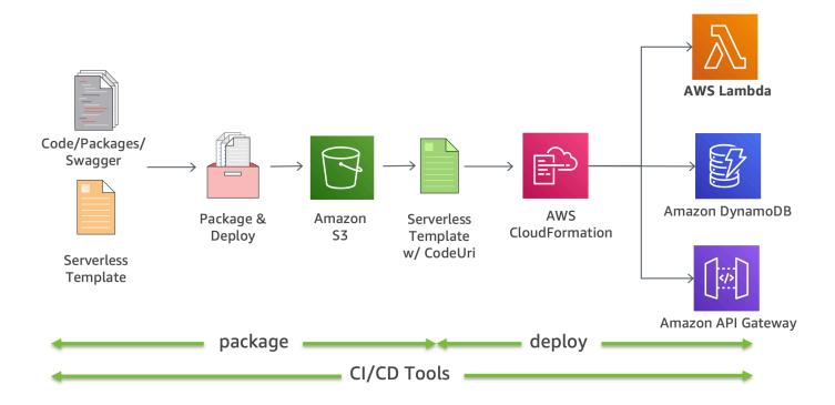
Figure 2: AWS Serverless Application Model (AWS SAM)
