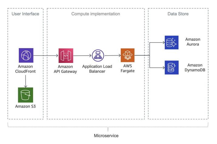
Figure 5: Serverless microservice using AWS Fargate
