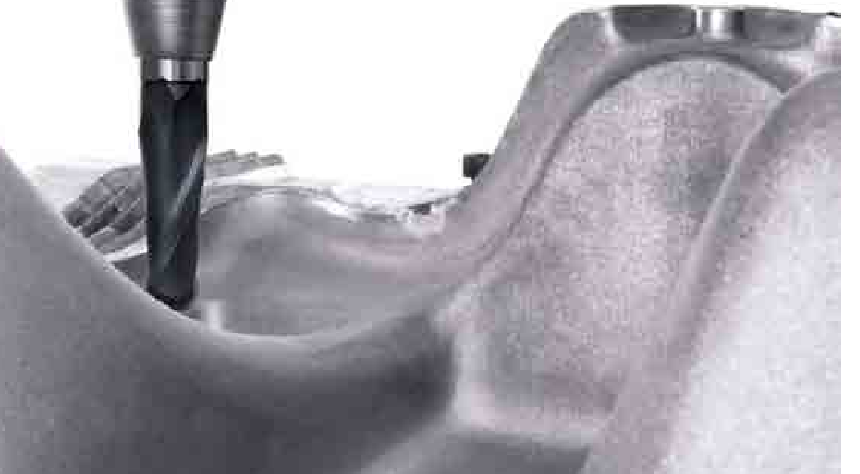
© INJECTION MOULD FROM TOOL STEEL FOR BOBBYCARS: completely manufactured in 45 hours on the DMC 105 v linear vertical machining centre with high-speed cutting with 90 m/min rapid traverses and up to 2g acceleration on all axes.
