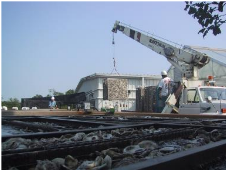
Figure 7 Stainless steel cages for high volume setting operation
