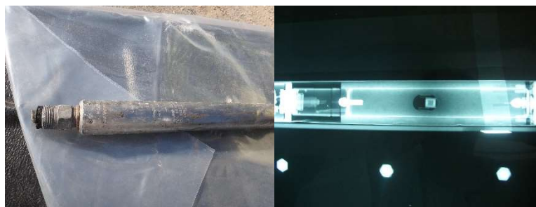
Fig.1: Ra-Be Source (At the arena on the left, Radiography on the right)
