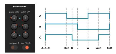
The pulsequencer is a generative module, which creates repeating complex melodies using nothing but three simple square LFOs which are synced to the current tempo.
