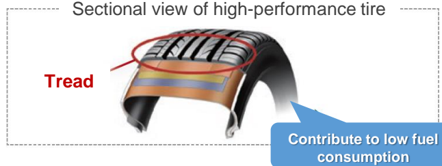
Sectional view of high-performance tire
