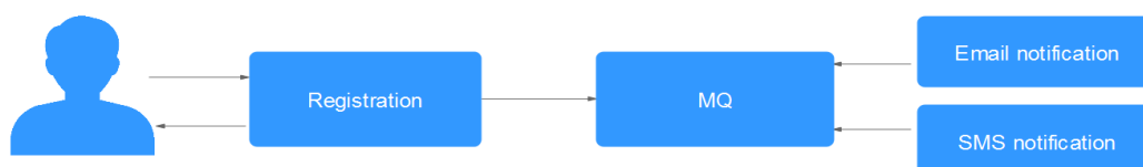
Figure 4-2 Asynchronous registration and notification using message queues
