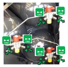
CNG automatic overpressure and overtemperature safety valves:
