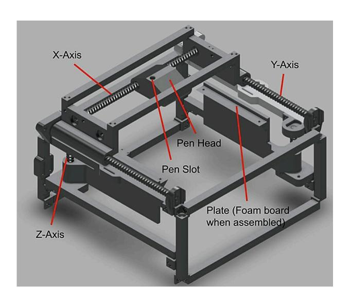
Labeled model of the system's frame, outlining the arrangement of components and its overall design. Credit: Tianyi Huang and Richard Xiong.
