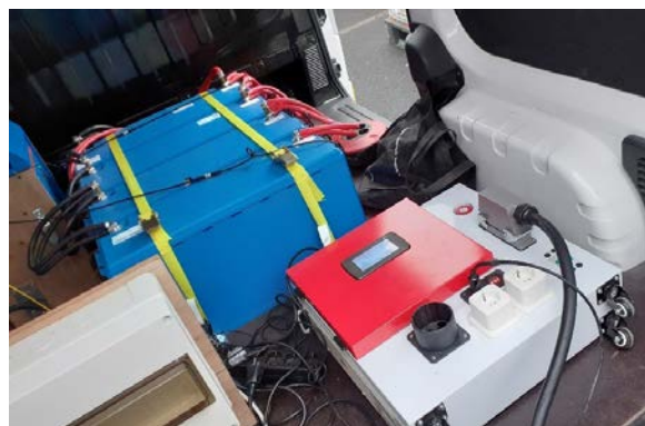
Figure 7: Bidirectional V2box charger/discharger (in red and white color), combined with a battery rack (in blue color)
