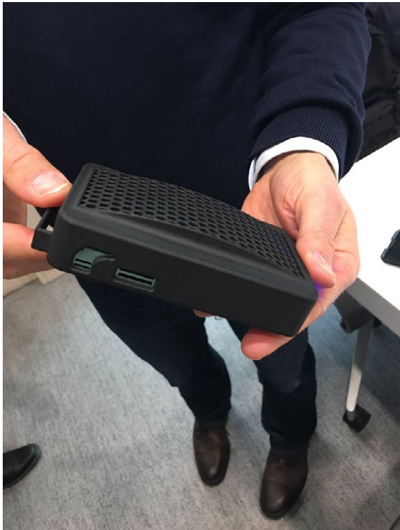
Figure 3: HOPE lower-cost sensor system unit for monitoring of fine and respirable particles ( PM_{2.5} and PM_{10} ), ozone, nitrogen dioxide, carbon monoxide, temperature, barometric pressure, humidity, light and motion. Source: the HOPE project.
