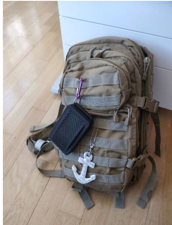
Figure 3: HOPE lower-cost sensor system unit for monitoring of fine and respirable particles ( PM_{2.5} and PM_{10} ), ozone, nitrogen dioxide, carbon monoxide, temperature, barometric pressure, humidity, light and motion. Source: the HOPE project.
