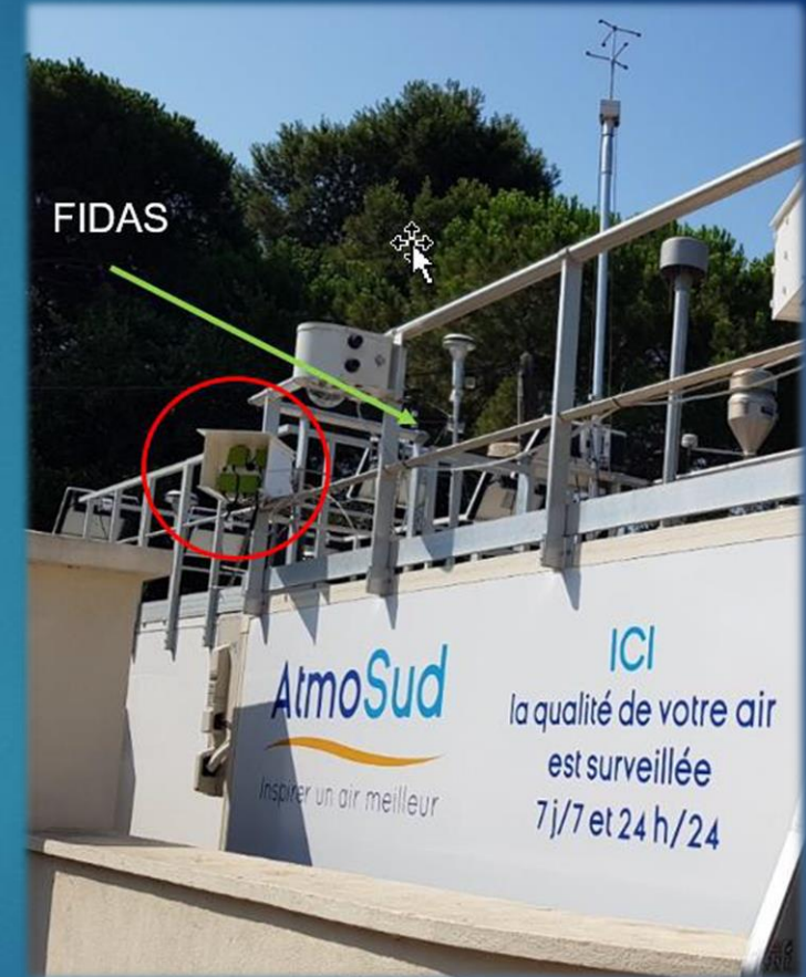
Collocation of the small sensors in one of the AtmoSud monitoring stations in Marseille. FIDAS is one of the EN approved instrument to measure particulate matter in the EU.
