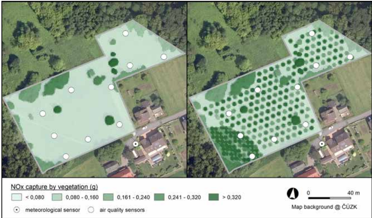
Capture of NO x (g) before the planting (on the left) and after the planting of the proposed vegetation (on the right) in a 1 x 1 m grid at the Radvanice site. Modelled for a two-month period (at the end of the growing season).
