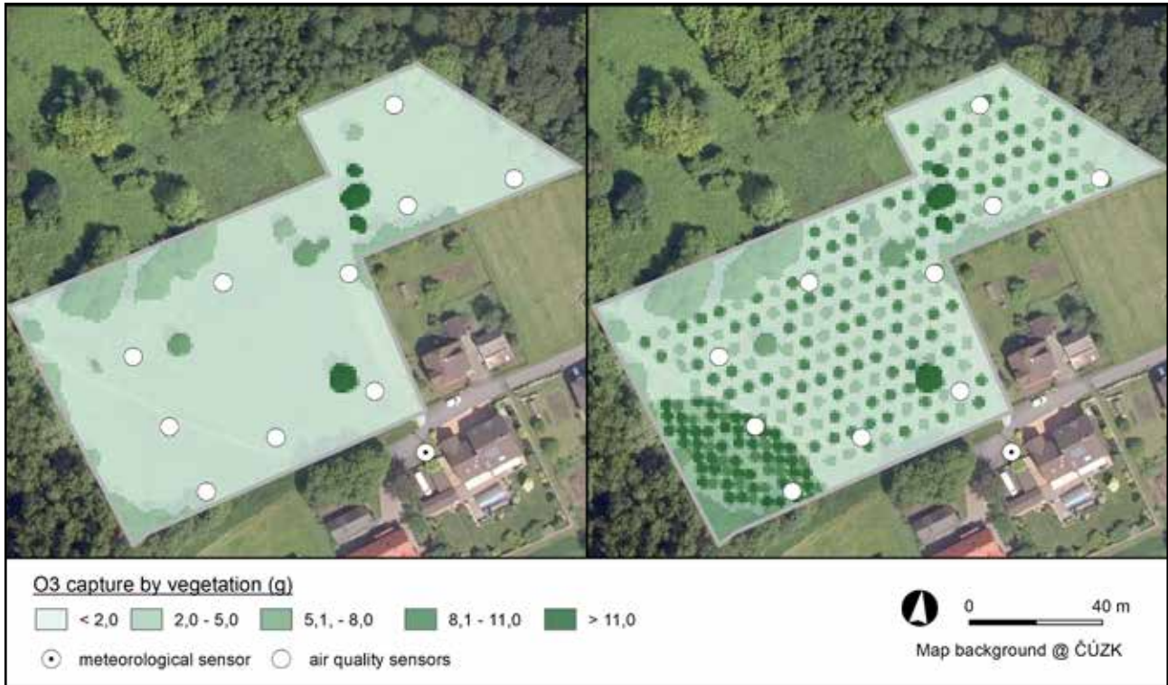
Capture of O 3 (g) before the planting (on the left) and after the planting of the proposed vegetation (on the right) in a 1 x 1 m grid at the Radvanice site. Modelled for a two-month period (at the end of the growing season).
