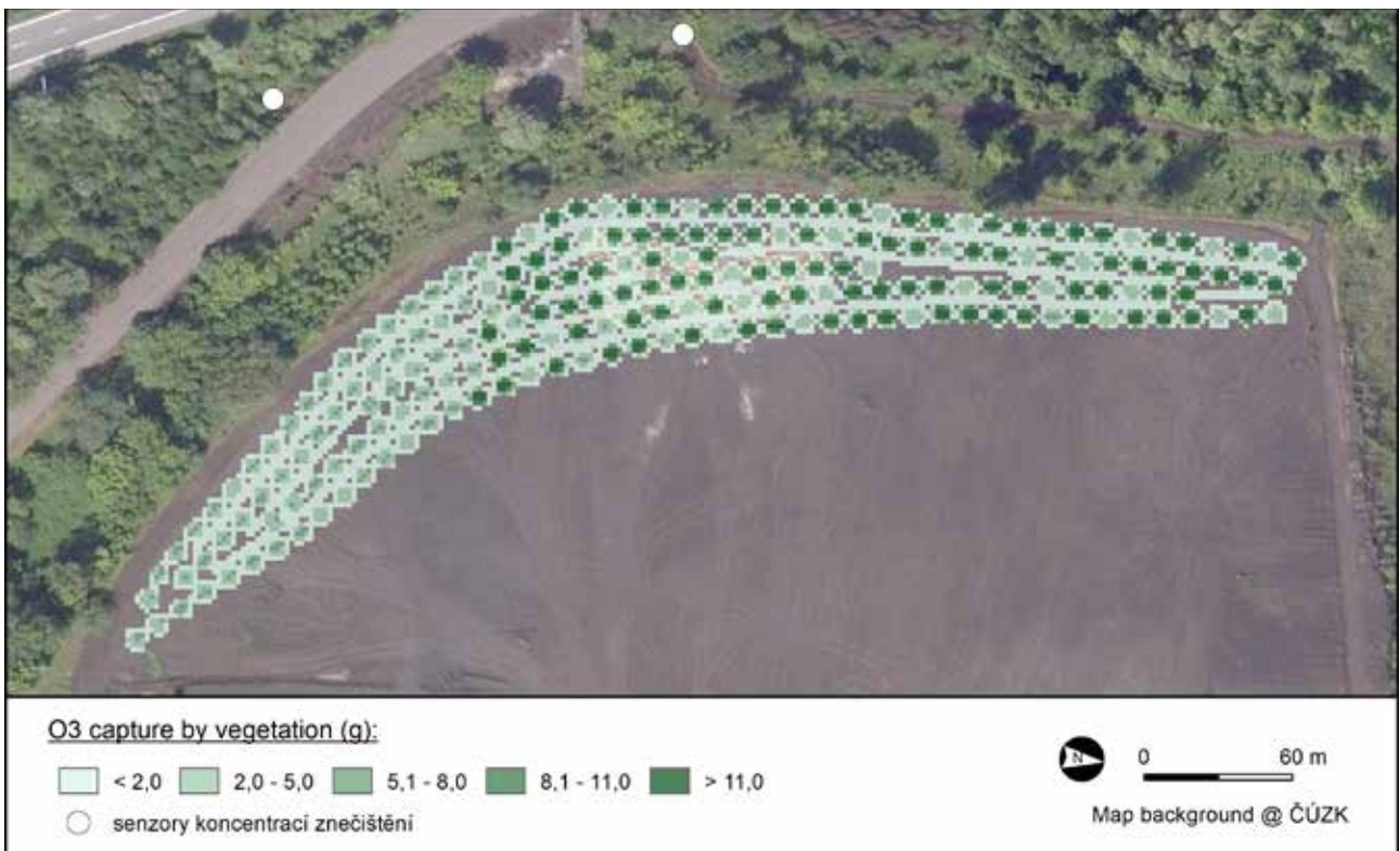
Fig. 15.6. Capture of O 3 (g) before the planting of the proposed vegetation in a 1x1 m grid at the Bartovice site. Modelled for a period of two months (at the end of the growing season). No significant capture is expected before the planting due to the absence of any current greenery.
