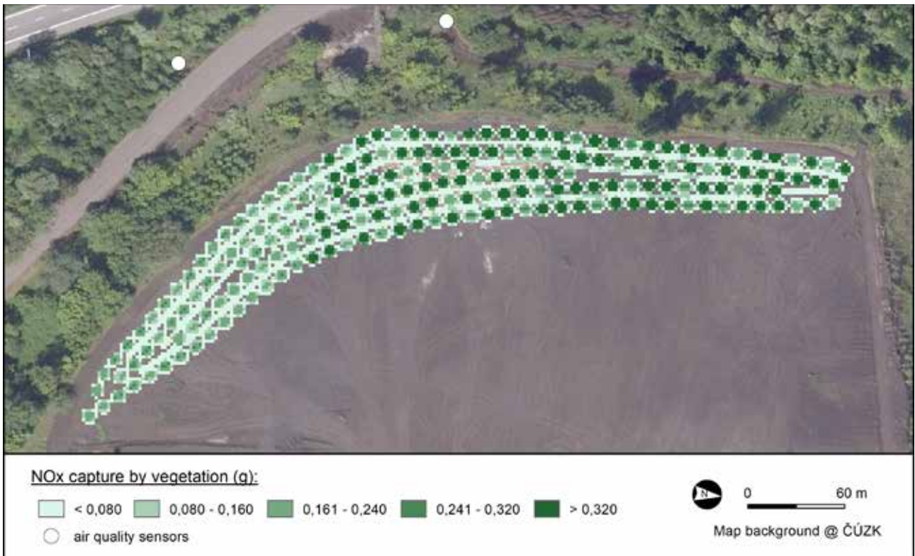
Fig. 15.8. Capture of NO_x (g) after the planting of the proposed vegetation in a 1 x 1 m grid at the Bartovice site. Modelled for a two-month period (at the end of the growing season). No significant capture is expected before the planting due to the absence of any current greenery.
