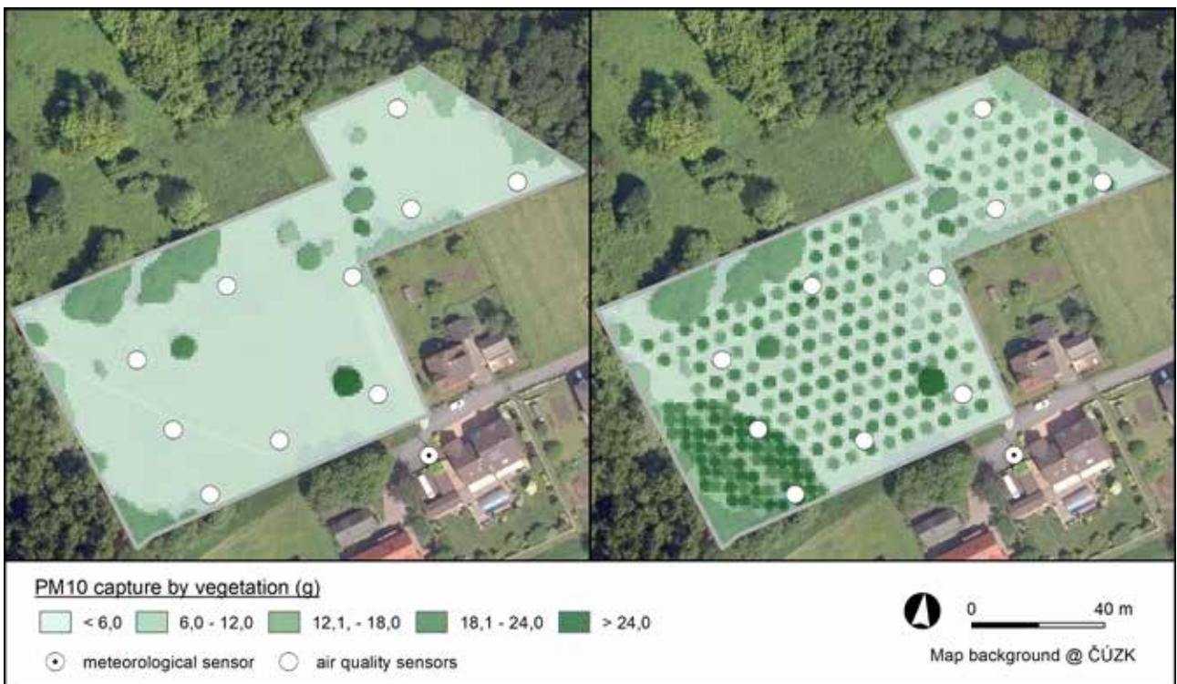
Fig. 15.4. Capture of PM 10 (g) before the planting (on the left) and after the planting of the proposed vegetation (on the right) in a 1x1 m grid at the Radvanice site. Modelled for a two-month period (at the end of the growing season).
