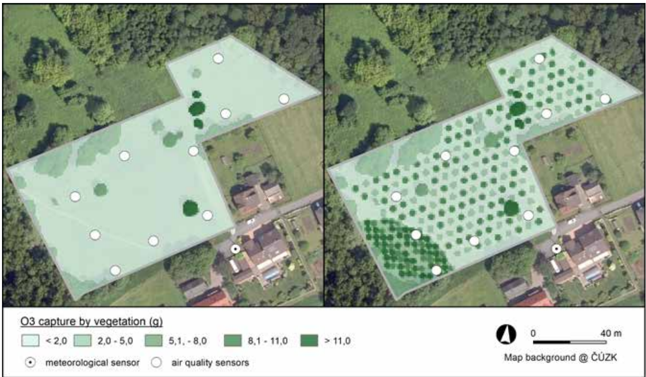
Fig. 15.3. Capture of O 3 (g) before the planting (on the left) and after the planting of the proposed vegetation (on the right) in a 1x1 m grid at the Radvanice site. Modelled for a two-month period (at the end of the growing season).
