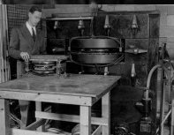
A larger push-button 25-MeV device, shown behind Kerst in the photo above, was built by the Allis-Chalmers Company and was used as an x-ray lithography device for detecting flaws in metals or other materials for the war effort.
