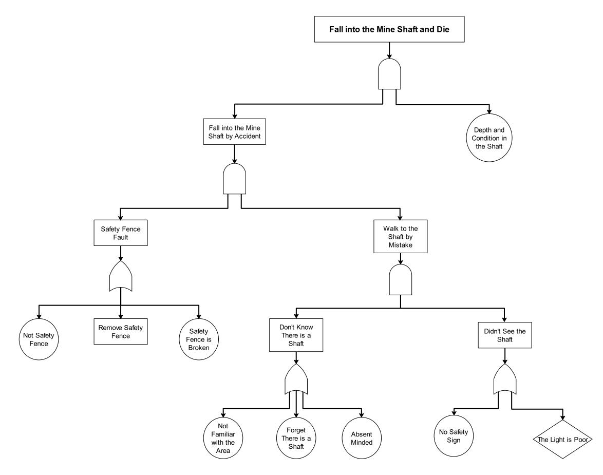
**Fault tree analysis** (FTA) is a top-down, deductive failure analysis in which a system's undesirable state is examined by combining a succession of lower-level occurrences using Boolean logic. This analysis method is mostly used in safety engineering and reliability engineering to quantify (or obtain a sense for) occurrence rates of a safety accident or a specific system level (functional) failure, as well as to discover the best ways to reduce risk.
