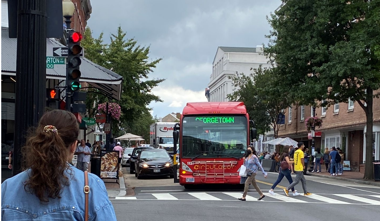
Figure 19: Bus Protruding the Travel Lane due to Unauthorized Vehicles Stopped in the Bus Zone
