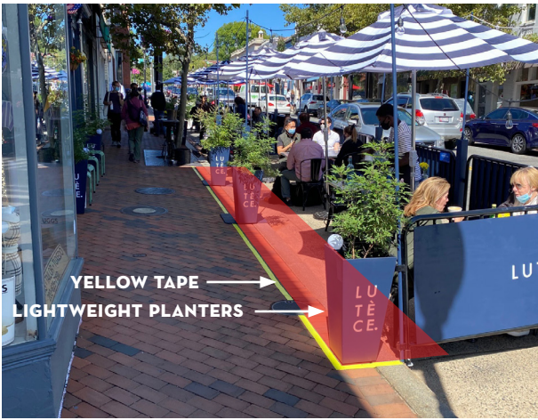
THE 4-FOOT BUFFER MUST BE CLEARLY DELINEATED AS SHOWN ABOVE WITH YELLOW TAPE AND MOVABLE PLANTERS.
