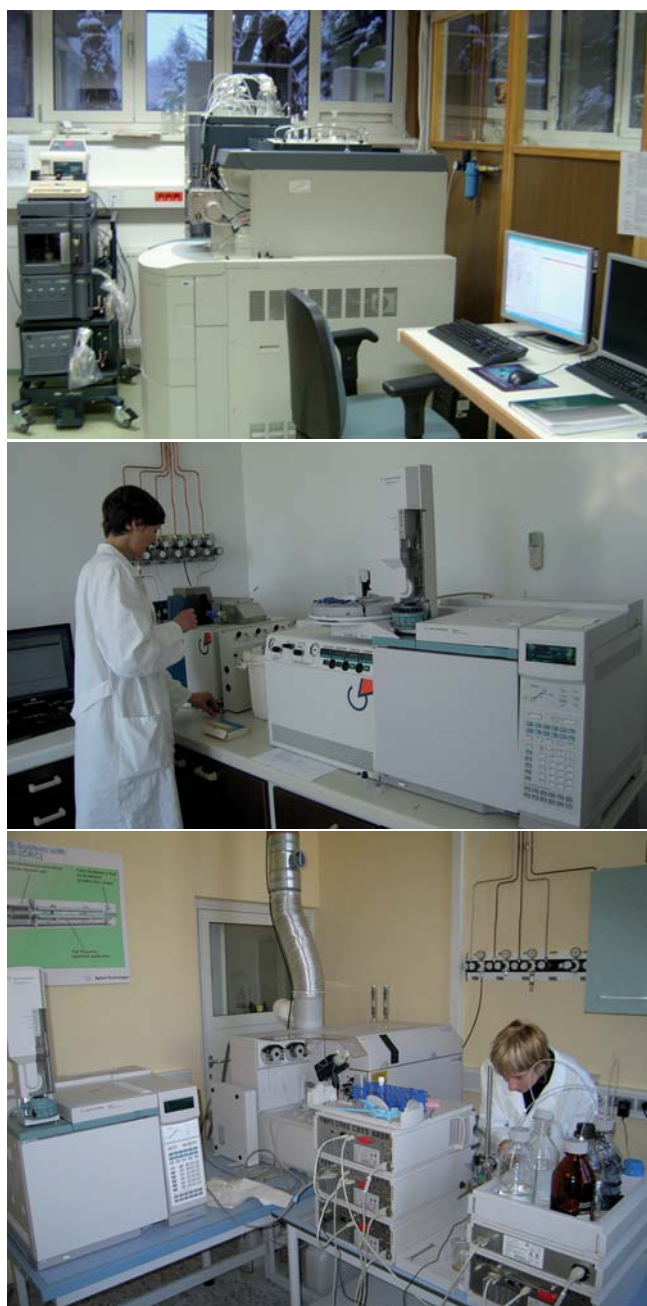
Figure 2: The department installed three mass spectrometers that will enlarge the spectrum of research in the area of biogeochemical cycling of substances in the environment, environmental technologies, and environment and health research projects: (1) Q ToF Premier with EI, MALDI, LC-MS, and MS-MS modes, (2) Compound-specific stable-isotope analyzer (IR-CS-MS) and (3) Inductively Coupled Plasma Mass Spectrometer (ICP-M) hyphenated with either HPLC or GC. The equipment was co-financed by European Structural Funds.
