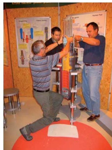
Figure 2: The mockup of the reactor pressure vessel is intended for specialists' training, but is also interesting for the general public
