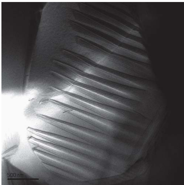
Figure 4: Bright-field STEM image of ferroelectric domains in a grain of BaTiO 3 -based PTC ceramics. Dept for Advanced Materials: B. Jančar.
