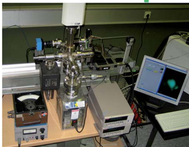
Figure 5: The principle of operation (above) and the complete setup for the control of the scanning projection field-emission microscope (below).
