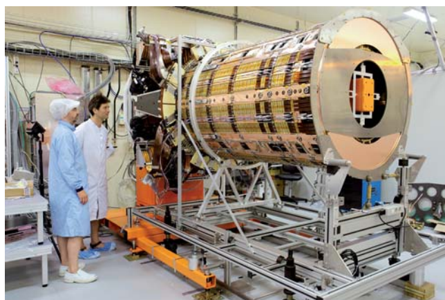
Figure 1: One of the two fully assembled ATLAS SemiConductor Tracker (SCT) end-caps ready for insertion into the Transition Radiation Tracker. On the cylinder's surface, flexible large-scale power tapes can be seen, which fan out from the detector in the rear. The tapes were produced in Slovenia as part of our contribution to the ATLAS construction.
