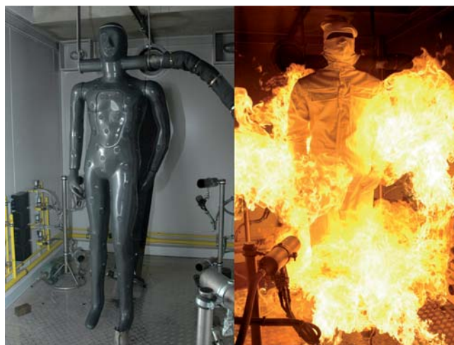
Figure 5: Testing of clothing to protect against fire using the flame manikin
