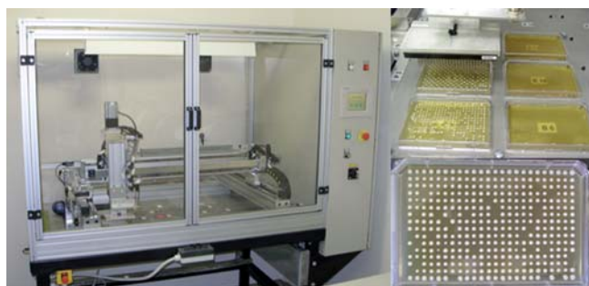
Figure 2: A new robot for the automatic replication of arranged colonies of microorganisms (yeast).
