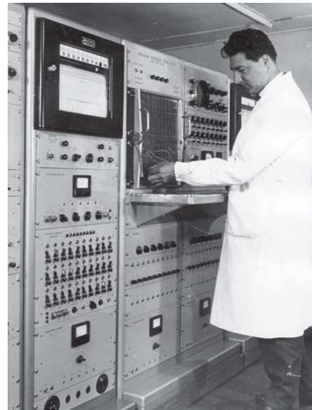
The M-2 analogue computer was designed and assembled at the JSI in 1959
