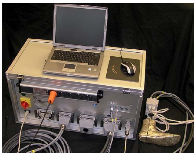
Figure 4: System for the evaluation of the thermal and evaporative characteristics of footwear
