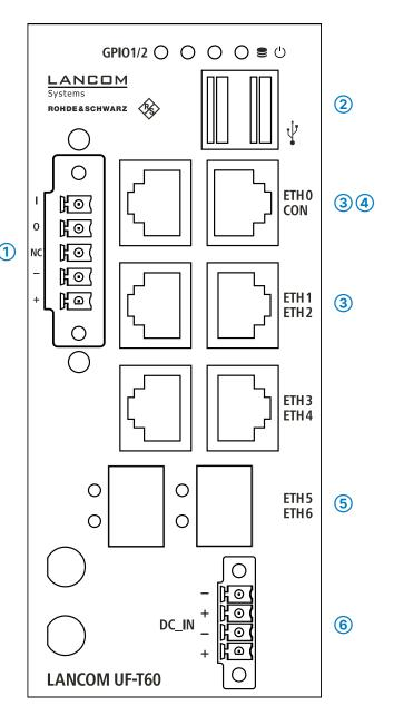
5-pin GPIO terminal block connector (TTL level) For connecting DIO\_PWR, DIO\_GND, GPO0, and GPIO
