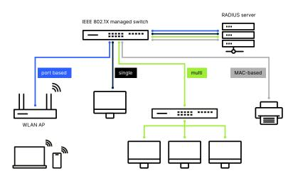
Figure 1: IEEE 802.1X — four methods of access control at a glance
