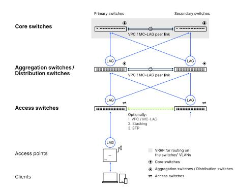
Figure 1: Three-tier network with redundancies
