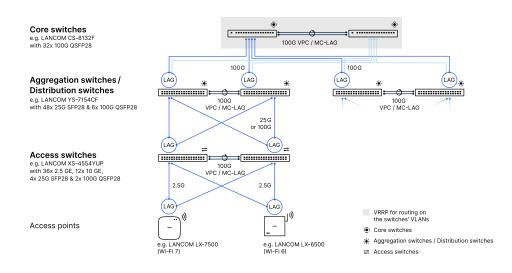
Figure 2: Scenario using VPC-capable access switches
