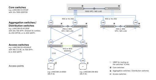
Figure 3: Scenario with a combination of VPC and stacking
