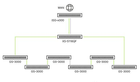
Figure 6: STP with numerous cascaded access switches
