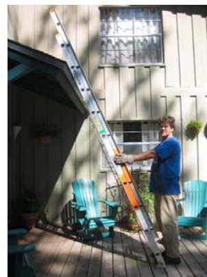
Proper angle of extension ladder
