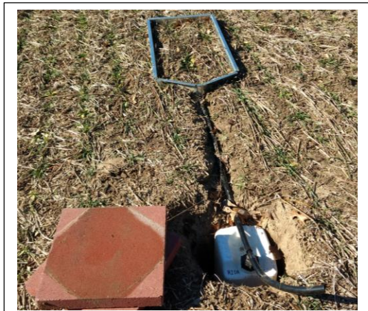
Figure 8. Example of 0.31 m 2 erosion weir installed in drilled rye cover crop plot in October. Site must have at least 5% slope for this apparatus to work effectively. The collection 8-liter (2 gal) jug is sized to collect all the runoff anticipated from a 5 cm (2 inch) storm.
