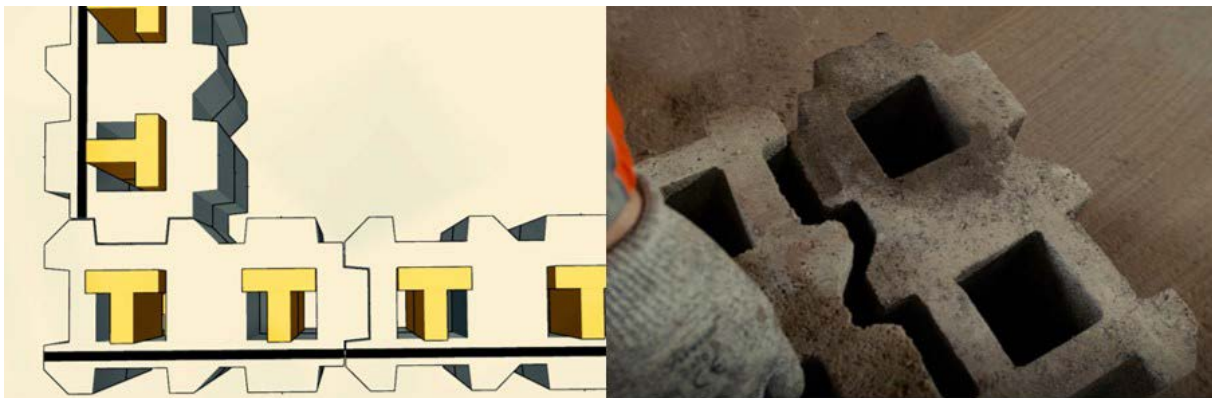
Figure 13: BRX design of connections left and one assembly option of BRX block right (developed by Pieter Sheer, Dusseldorp 2020)
