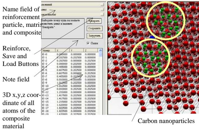
Fig. 5. Reinforced nanocomposite: metal matrix – carbon-based nanoparticles
