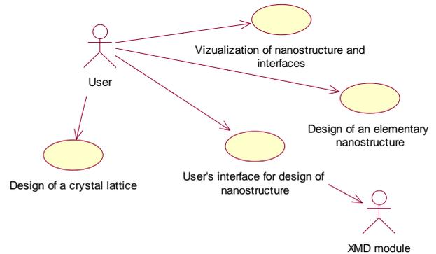
Fig. 2. "Use case" diagram for CAD/CAM of nanostructures
