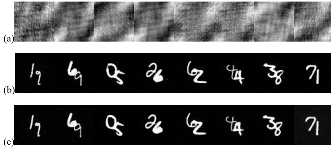
Fig.4 Test result of the media of same property dataset : (a) speckle image; (b) original target; (c) output image of PDSNet.
