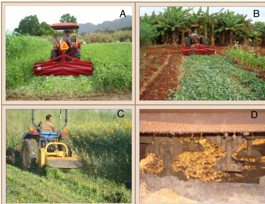
Fig 2. Roller crimper (A, B) is used at experiment stations at the University of Hawai'i to terminate various tropical legumes for no-till practice. Farmers often own a flail mower (C) to chop up crop residues above soil level (D) (photo credit: K.H. Wang).
