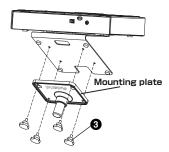
Fasten the mounting plate to the PSD-10.
