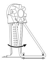
3. Use a tuning key to tighten the screws removed in Step 1 so that the stand is firmly secured.
