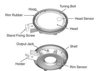
\* Do NOT place your fingers inside the shell, as you may hurt yourself or cause damage to the PDX-8. Or when changing the head, do NOT touch any of the internal parts. Also, do not insert your fingers into the hole of the mounting bracket.
