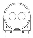
Position the two beaters equally apart from the center of the pad as shown in the figure at left. If one of the beater is further away from the center than the other, the sound from the further beater will be lower in volume, or will not sound as desired.
