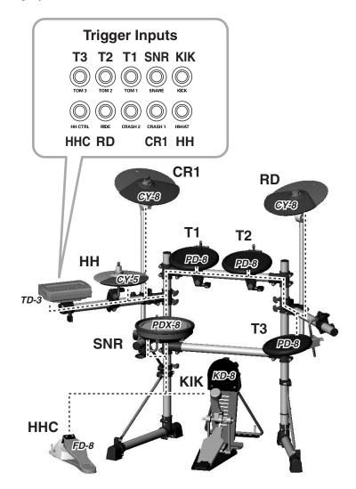
1. Insert the plugs of connecting cables into the TRIGGER INPUTS jacks on the rear of the TD-3.
