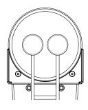
Position the two beaters equally apart from the center of the pad as shown in the figure at left. If one of the beater is further away from the center than the other, the sound from the further beater will be lower in volume, or will not sound as desired.
