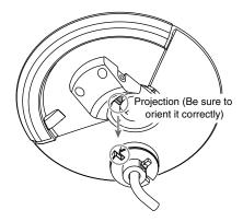
3. Place the clutch felt (s), and while applying some pressure, mount the upper clutch as shown.
