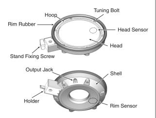
\* Do NOT place your fingers inside the shell, as you may hurt yourself or cause damage to the PDX-8. Or when changing the head, do NOT touch any of the internal parts. Also, do not insert your fingers into the hole of the mounting bracket.
