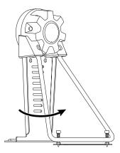
3. Use a tuning key supplied with the FD-8 to tighten the screws removed in Step 1 so that the stand is firmly secured.
