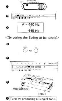
How to check a tone with Meter and Tuning Guide
